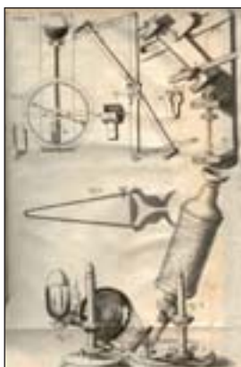
Robert Hooke's compound microscope.
